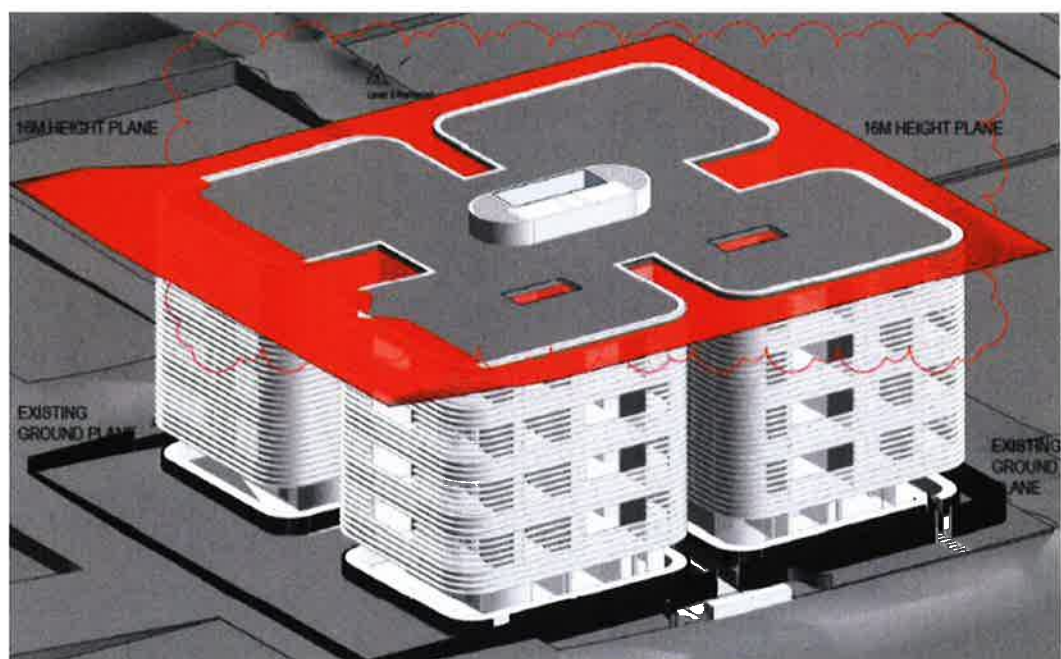
Figure 7. Height limit as depicted by the red area and shown in 3-dimensions, showing the non-compliant aspects of the proposal.
